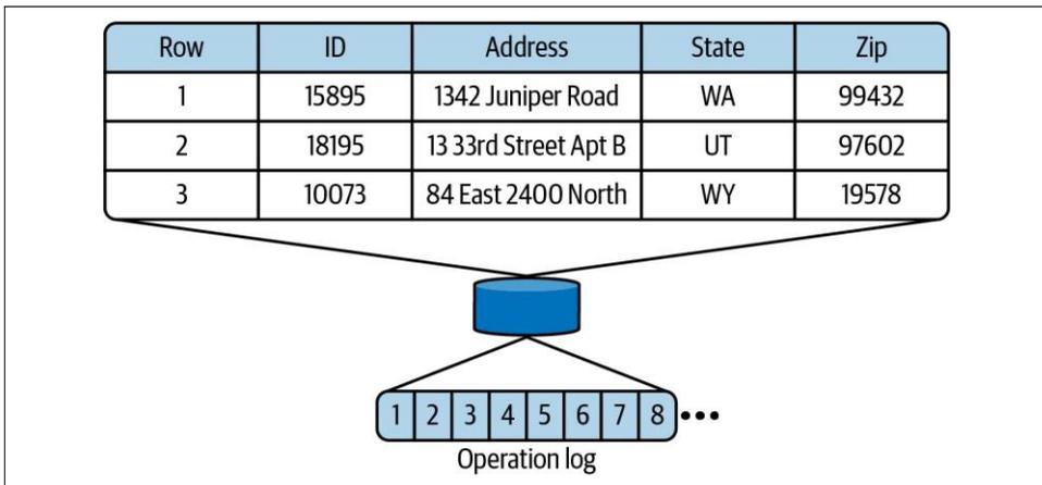
Figure 5-3. Database logs record operations on a table
