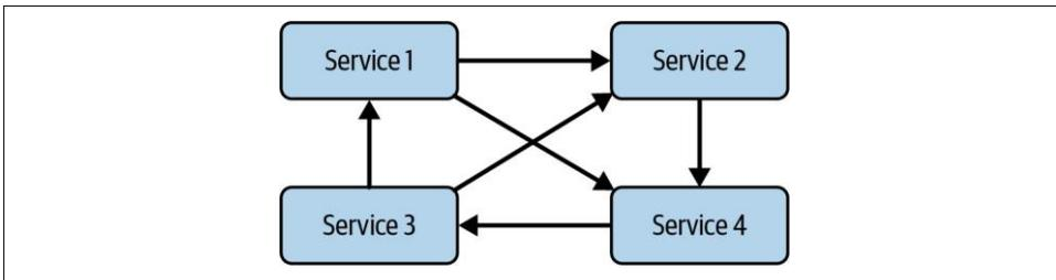
Figure 4-4. The monolith tightly couples its services
