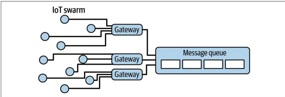
Figure 3-16. A device swarm (circles), IoT gateways, and message queue with messages (rectangles within the queue)
