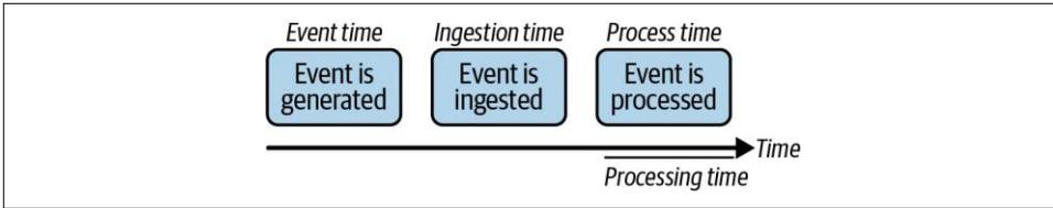
Figure 5-6. Event, ingestion, process, and processing time
