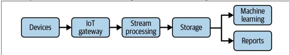
Figure 3-17. IoT serving pattern for downstream use cases
