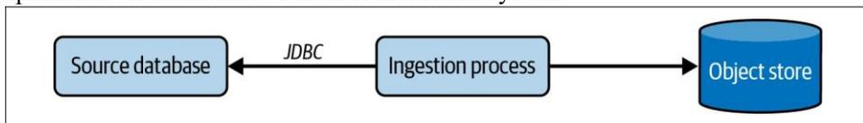
*Figure 7-13. An ingestion process reads from a source database using JDBC, and then writes objects into object storage. A target database (not shown) can be triggered to ingest the data with an API call from an orchestration system.*
