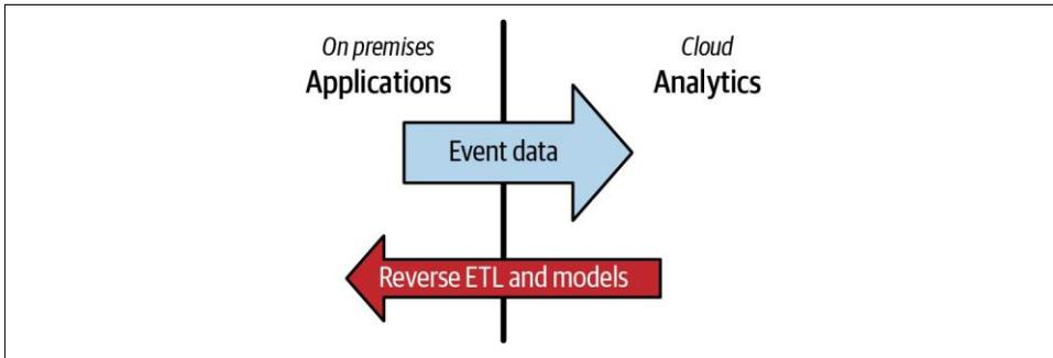
Figure 4-3. A hybrid cloud data flow model minimizing egress costs
