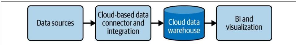
Figure 3-13. Basic components of the modern data stack
