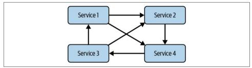
Figure 4-4. The monolith tightly couples its services
